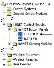
• The system tree of the control system displays the device in the appropriate slot with a default MNET ID as shown in the following illustration.
