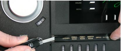
3. Continue sliding the screwdriver behind the label strip until the top of the label strip slides out as shown below.
